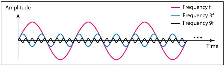
a. Time-domain decomposition of a composite signal
