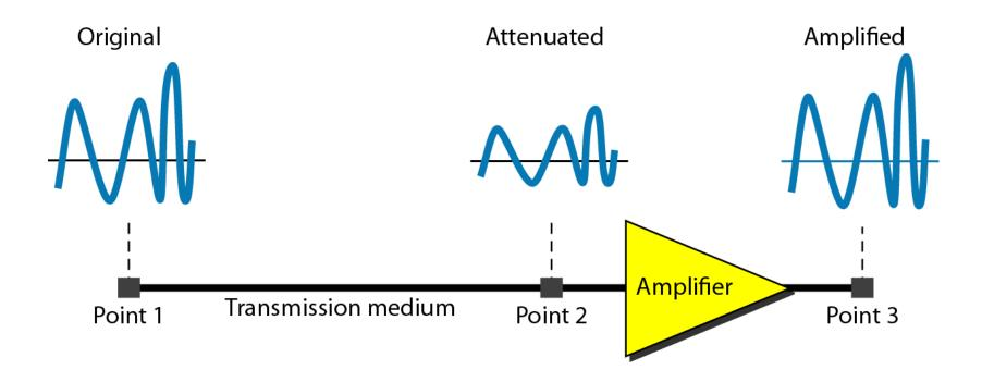
Suppose a signal travels through a transmission medium and its power is reduced to one-half. This means that  $P_2$ is  $(1/2)P_1$ . In this case, the attenuation (loss of power) can be calculated as
