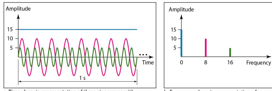
a. Time-domain representation of three sine waves with frequencies 0, 8, and 16
