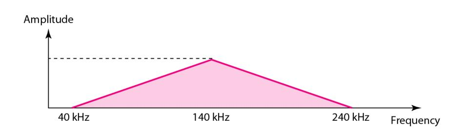
An example of a nonperiodic composite signal is the signal propagated by an AM radio station. In the United States, each AM radio station is assigned a 10-kHz bandwidth. The total bandwidth dedicated to AM radio ranges from 530 to 1700 kHz. We will show the rationale behind this 10-kHz bandwidth in Chapter 5.
