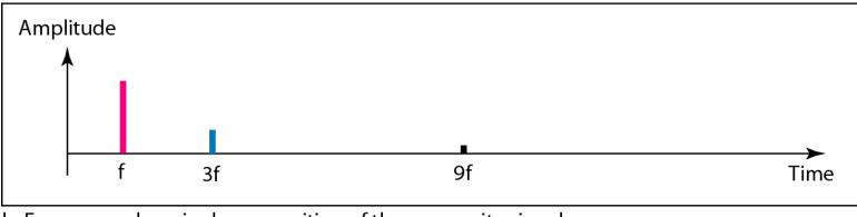
b. Frequency-domain decomposition of the composite signal
