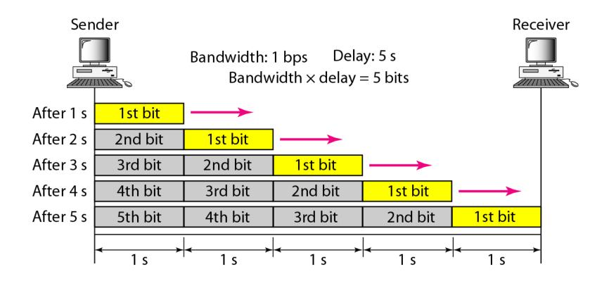
We can think about the link between two points as a pipe. The cross section of the pipe represents the bandwidth, and the length of the pipe represents the delay. We can say the volume of the pipe defines the bandwidth-delay product, as shown in Figure 3.33.
