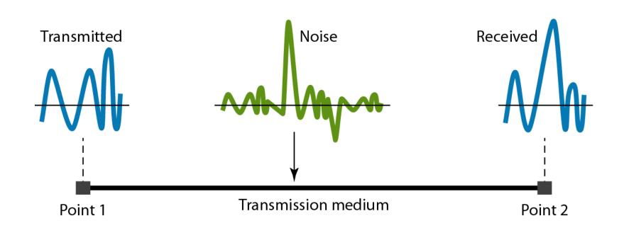
The power of a signal is 10 mW and the power of the noise is 1  $\mu$ W; what are the values of SNR and SNR<sub>dB</sub>?
